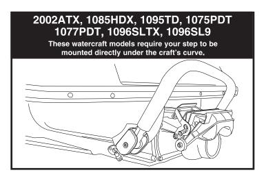
★ If you have the following step models:P/N 1075PDT, 1077PDT, 1085HXD, 1095TD, 2002ATX, 1096SLTX or 1096SL9, please note the special instructions while installing your step.
