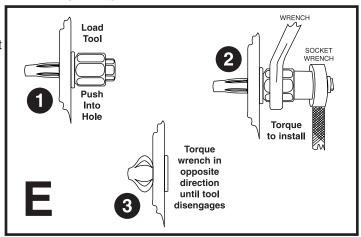
wrench clockwise. Once finished, remove installation tool by torquing counter clockwise. Do this same operation for all six holes. **SEE FIG. E**
