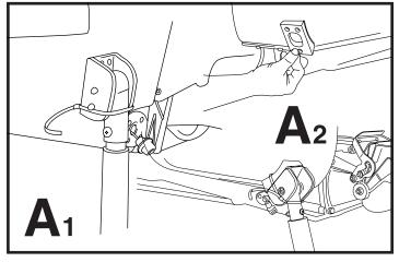
Center the step on the hull of the craft, finding the lowest location where your step can be centered. If your craft has a drain plug, center step above the drain plug, (you may mark the exact center of your craft, then measured to both sides of that mark to reassure your center)
